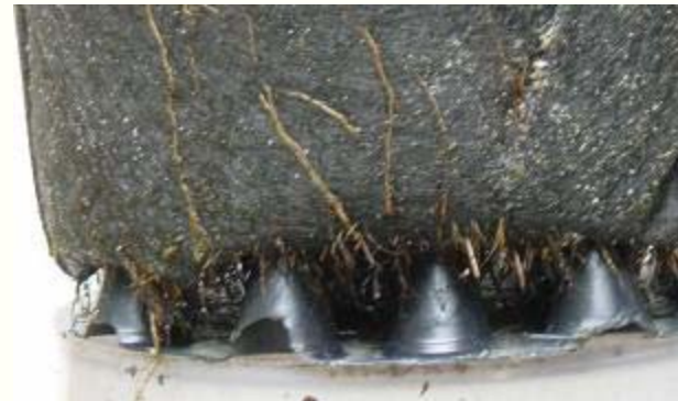
Filter fabric without 'root barrier'.
